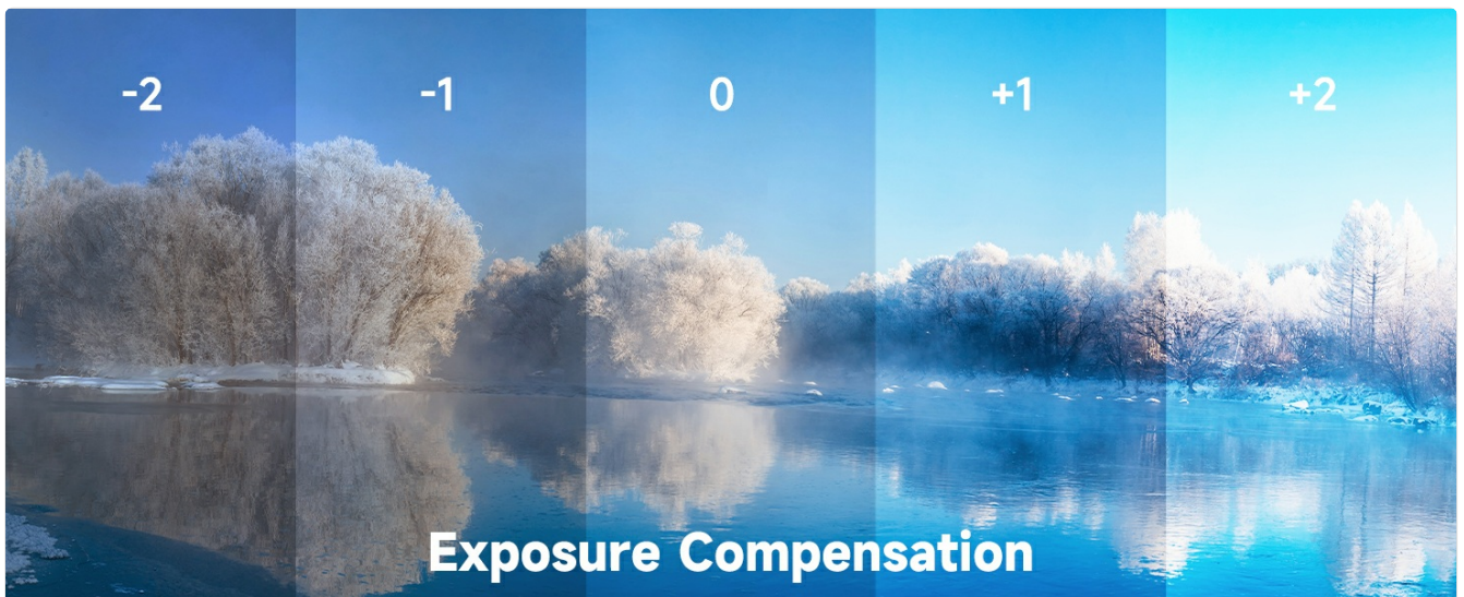
Figure 9: Visual representation of exposure compensation, showing how different settings affect image brightness.
