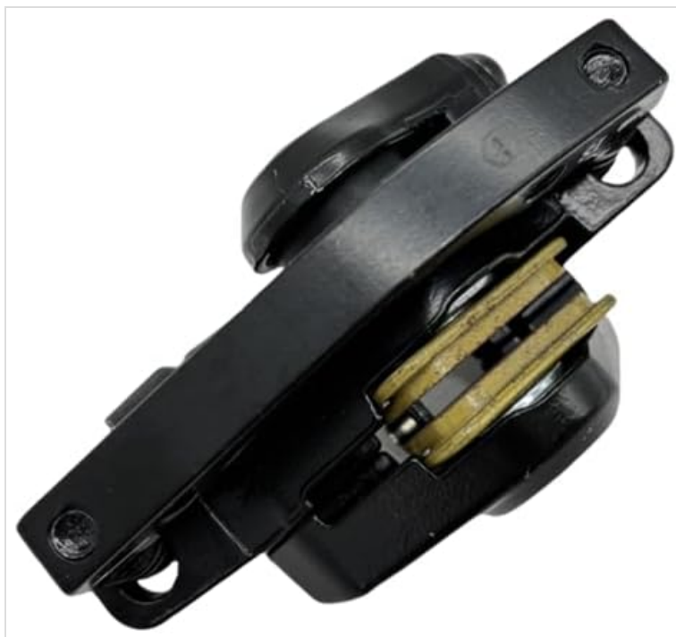
Figure 2: Bottom view of the caliper, highlighting the brake pads and their position within the caliper body.
