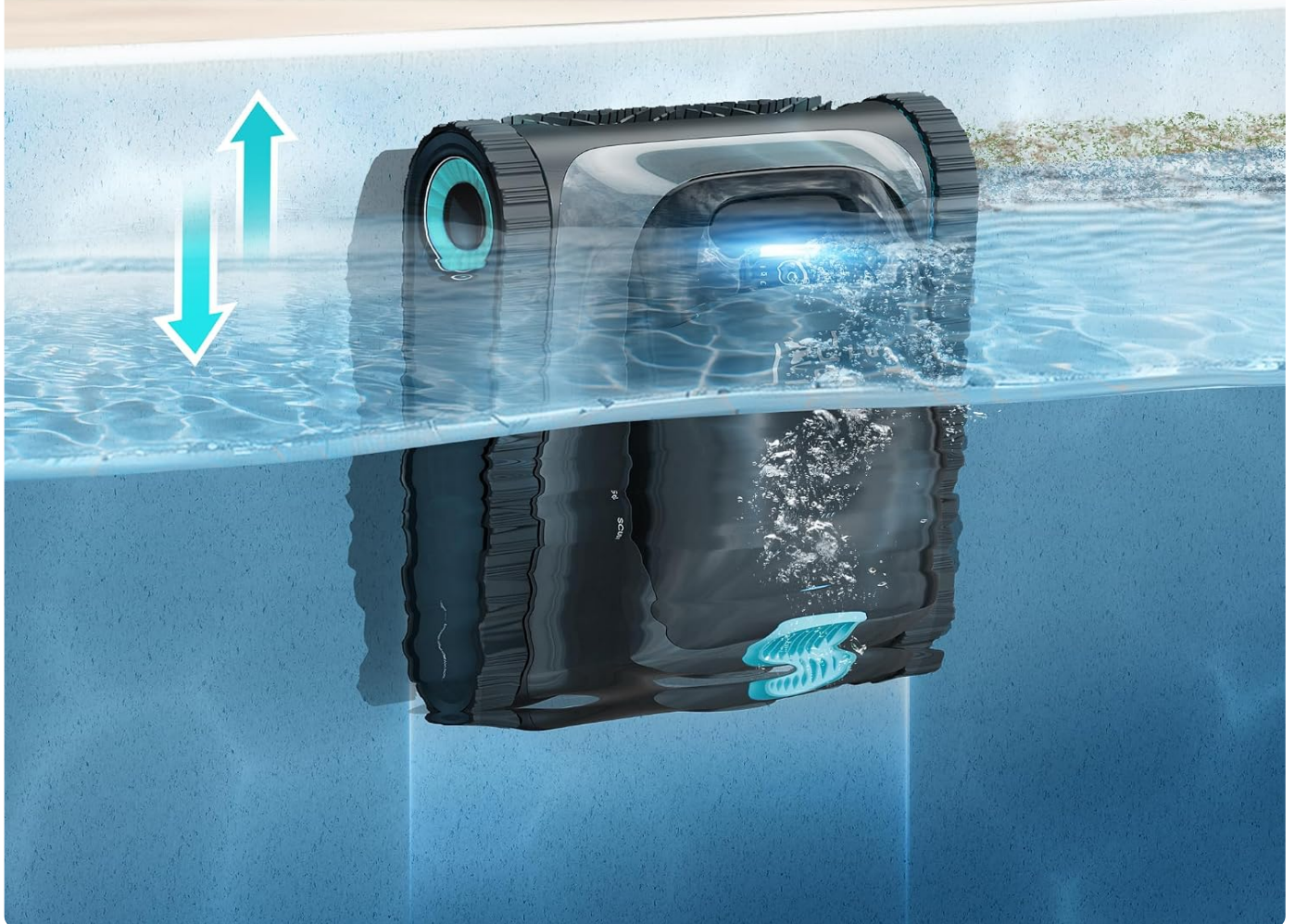
The Scuba S1 performing wall and waterline cleaning.
