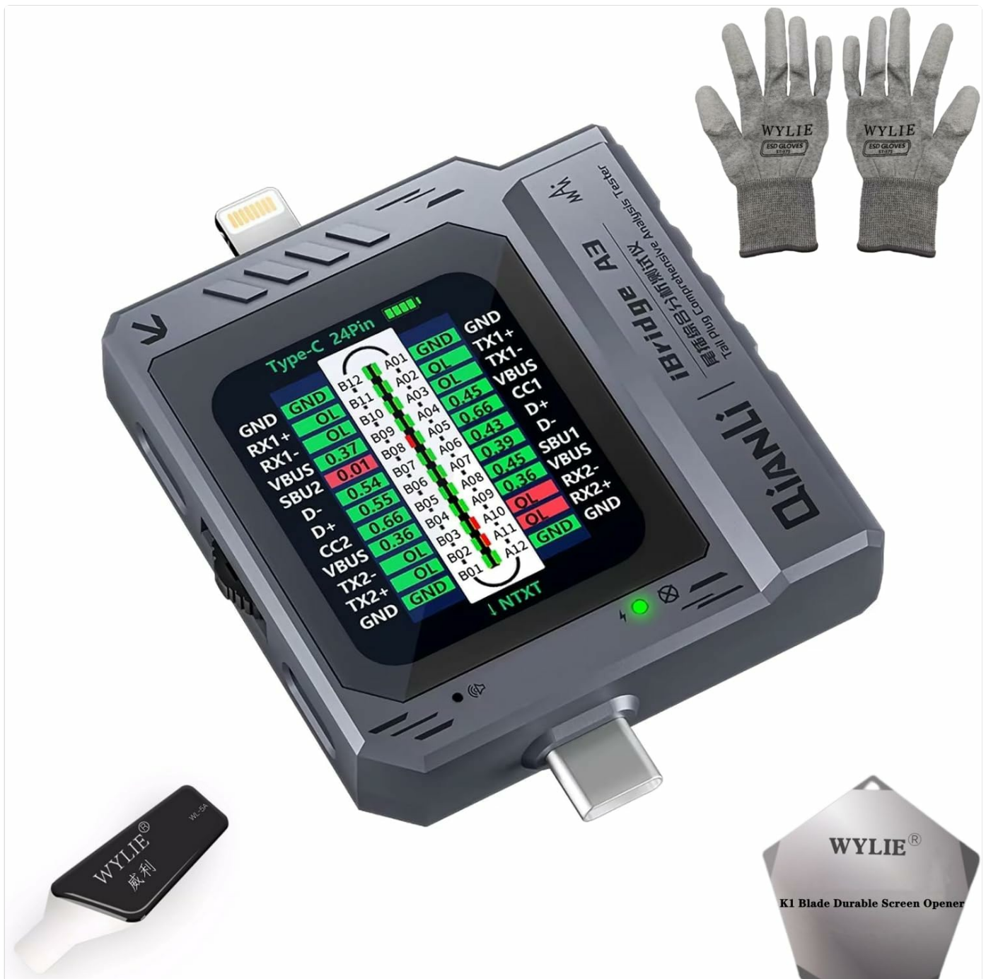
Image: The Qianli iBridge A3 Digital Tester shown with its accompanying accessories, including ESD gloves and a screen opener tool.
