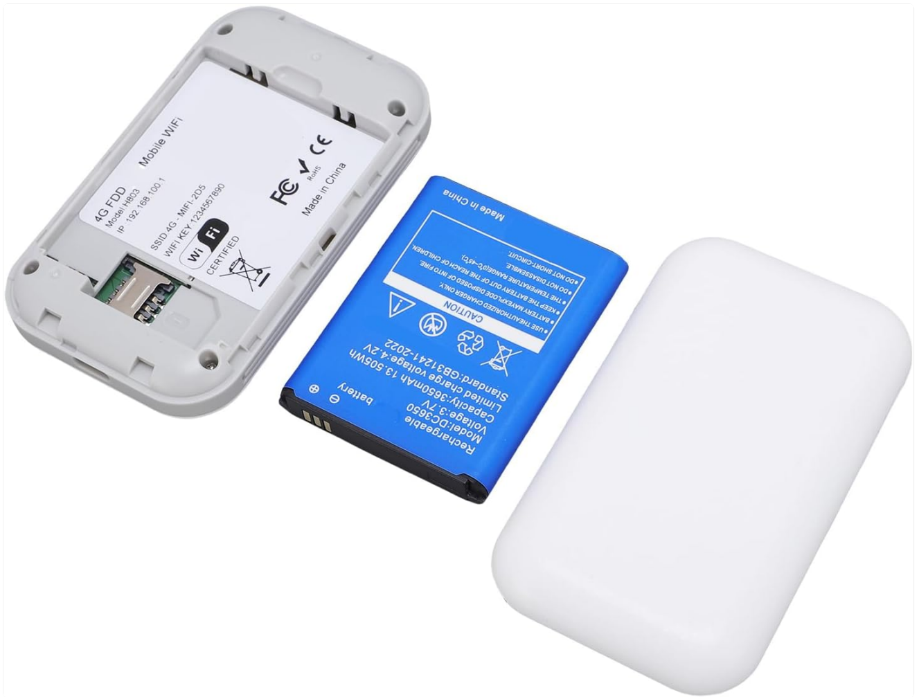
Image: The Bewinner Mobile Hotspot with its back cover and battery removed, revealing the SIM card slot.
