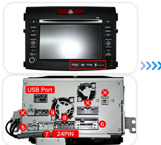
Image: Connection diagram for CAN020-R harness.
