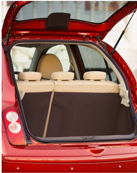
Image: A red car with its trunk open, illustrating the function of lift supports in holding the tailgate.
