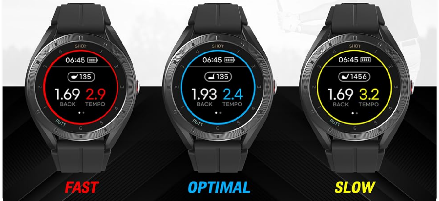
Image: The T11 LT Golf Watch displaying the Tempo Practice Mode with visual feedback for fast, optimal, and slow swing tempos.
