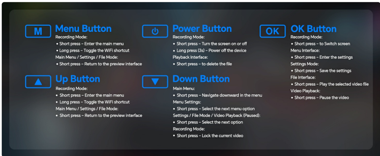
Image 5.1: Detailed explanation of each button's function in different modes (Recording, Menu Interface, Settings, File Interface, Video Playback).
