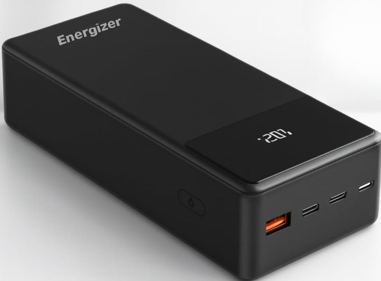
A front-angle view of the Energizer UE27062PQ Power Bank, showcasing its sleek black design, digital LED display, and the USB-A and USB-C output ports on the side.
