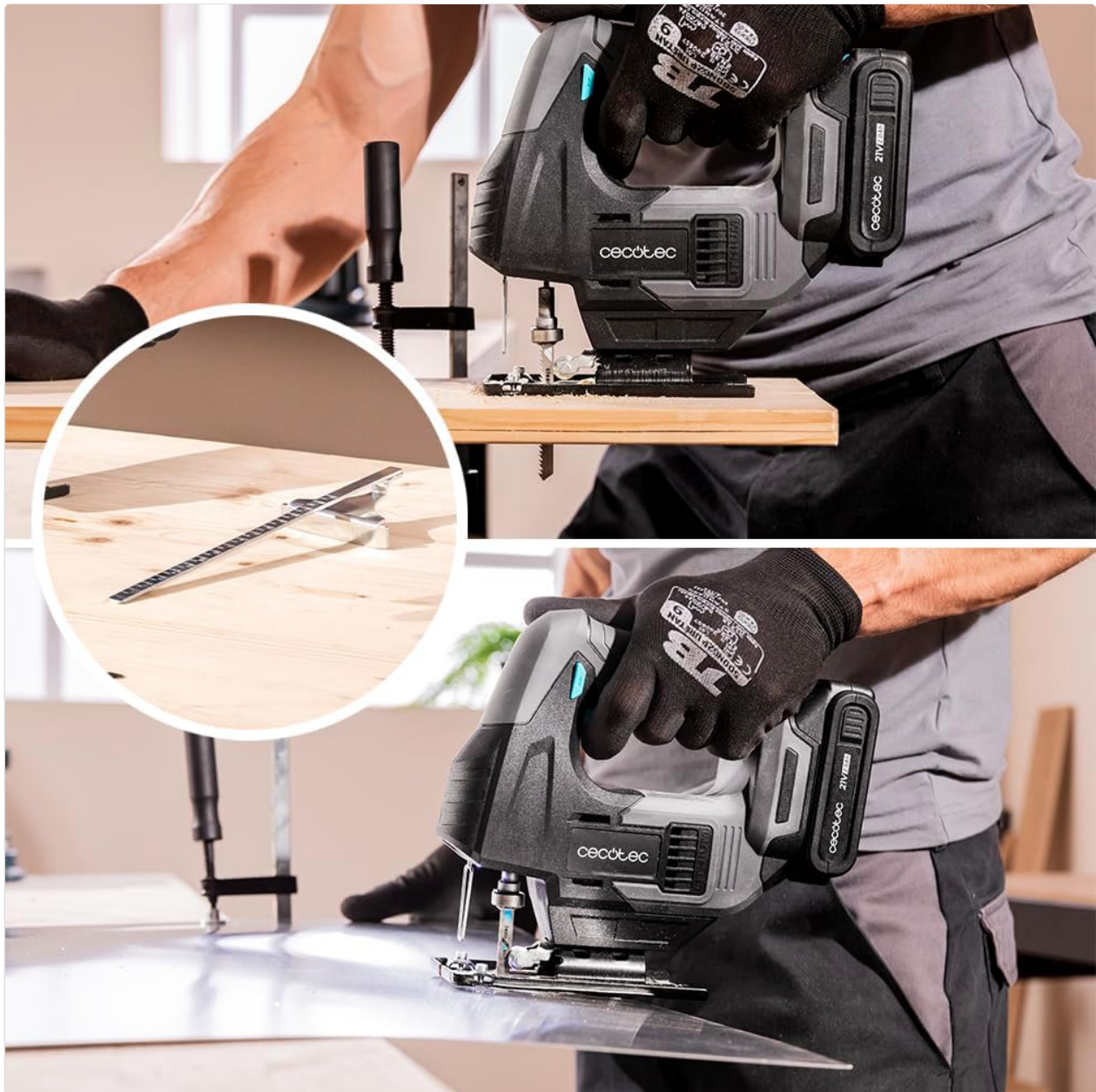
Figure 6: The jigsaw is capable of cutting both wood and metal with appropriate blades.
