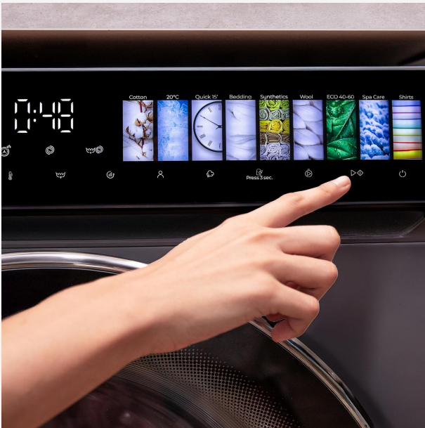
Figure 4.2: FullColor touchscreen control panel for program selection.
