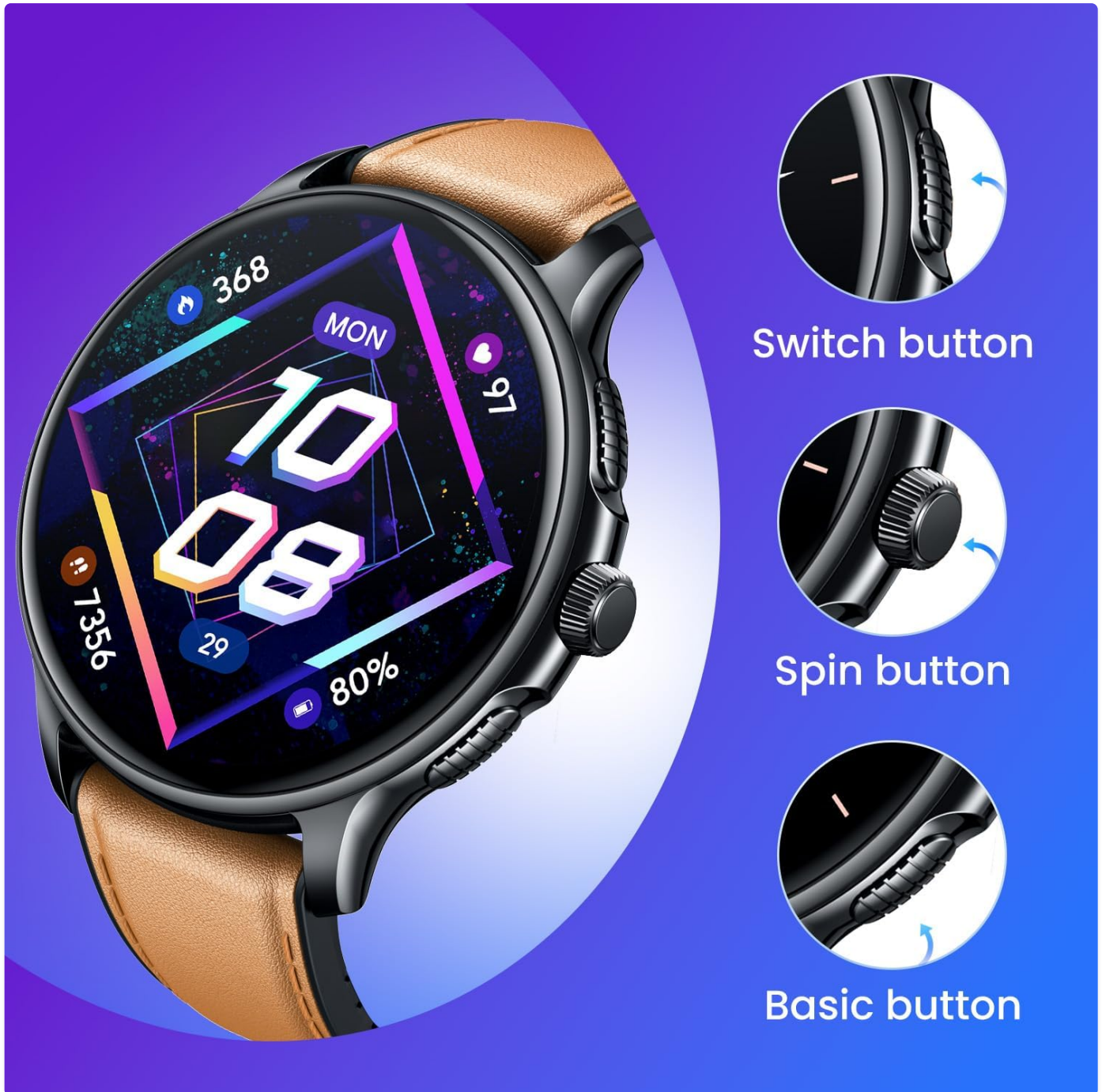
Image 4.1: Illustration of the smartwatch's physical controls, including the 'Switch button' for power and screen on/off, the 'Spin button' for menu navigation and selection, and the 'Basic button' for quick access or return functions.
