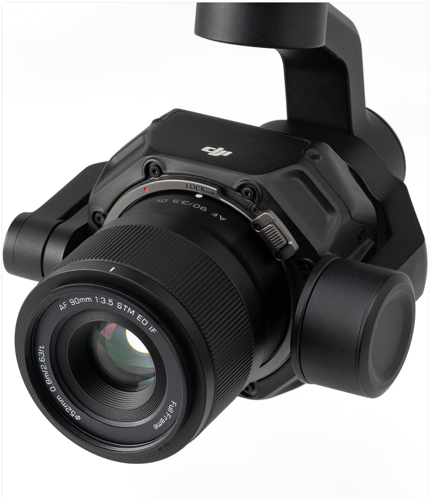
Figure 5.2: The VILTROX 90mm F3.5 DL lens securely mounted on a DJI gimbal, ready for operation.
