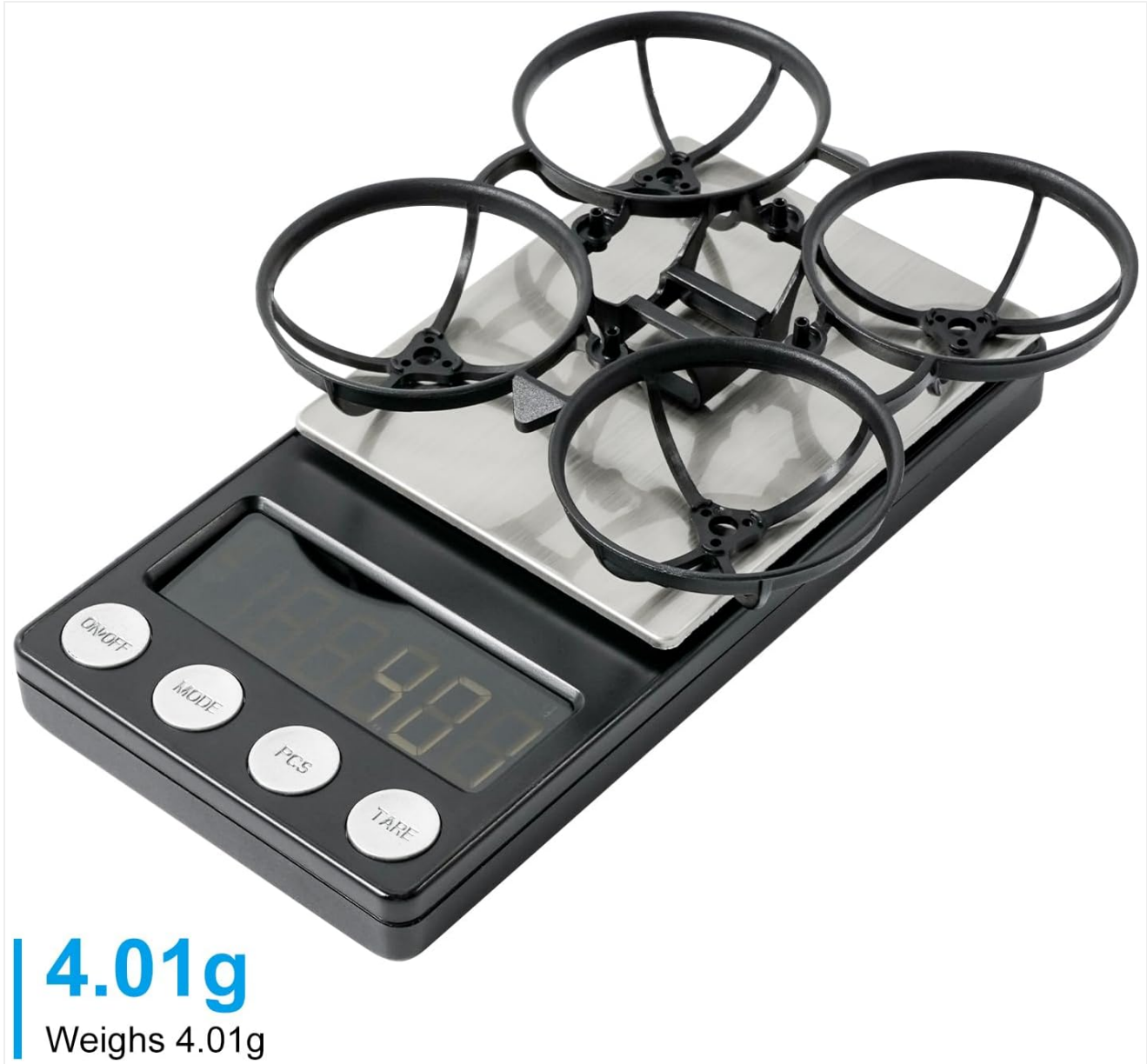
Figure 6: The Air75 II frame's ultra-light weight of 4.01g.
