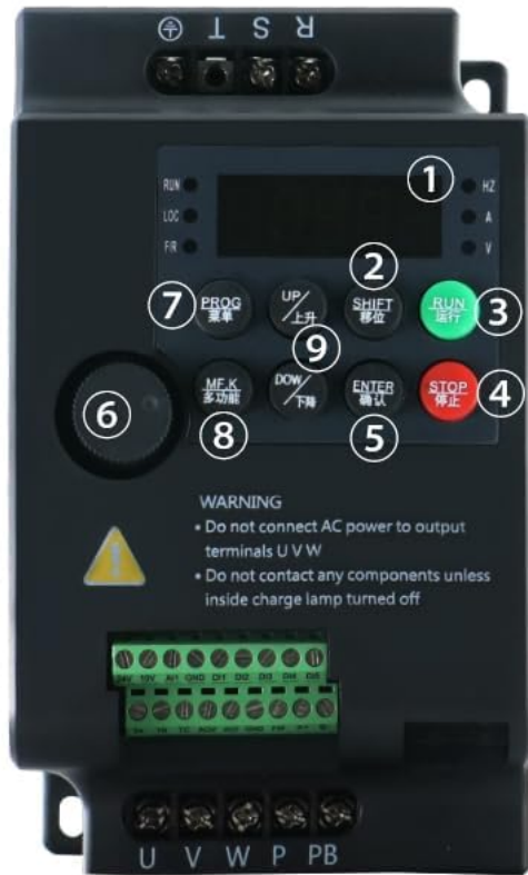
Figure 2.3: Detailed diagram illustrating the function of each key on the VFD's control panel.
