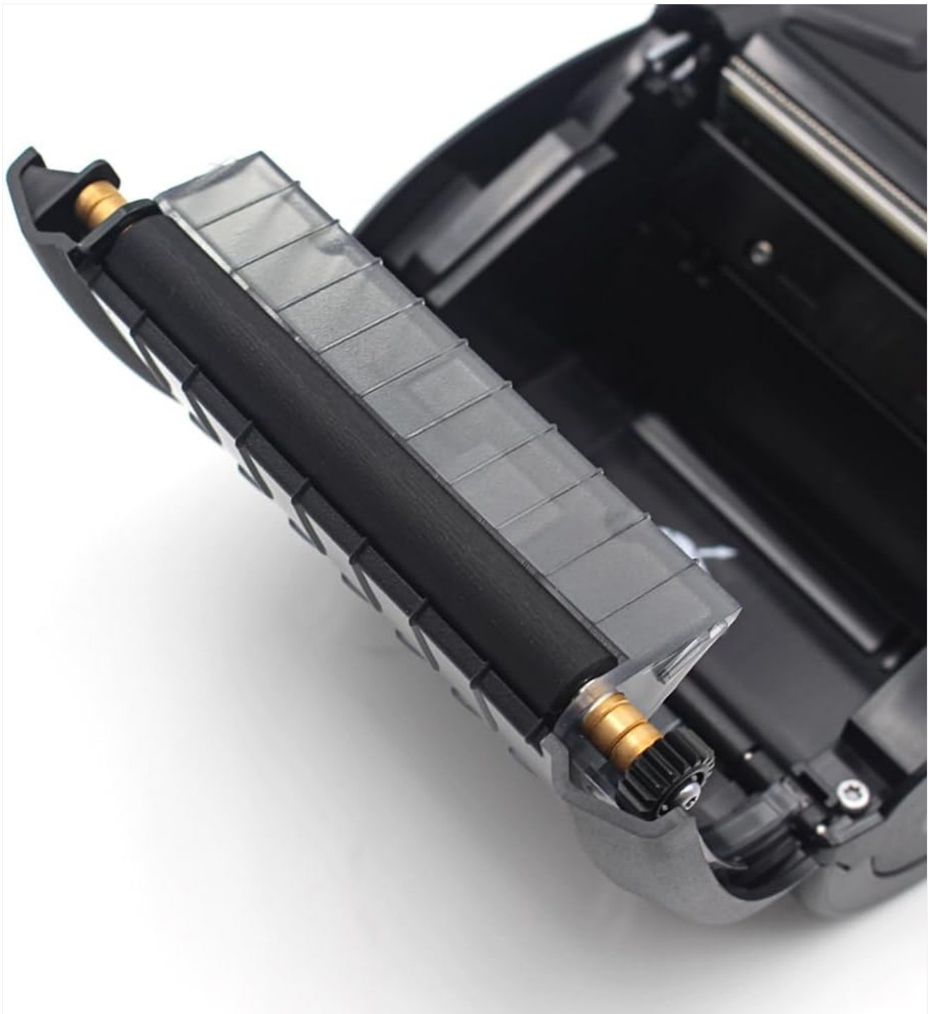
Figure 5: Close-up of the ZQ220 print roller and mechanism, which should be kept clean.
