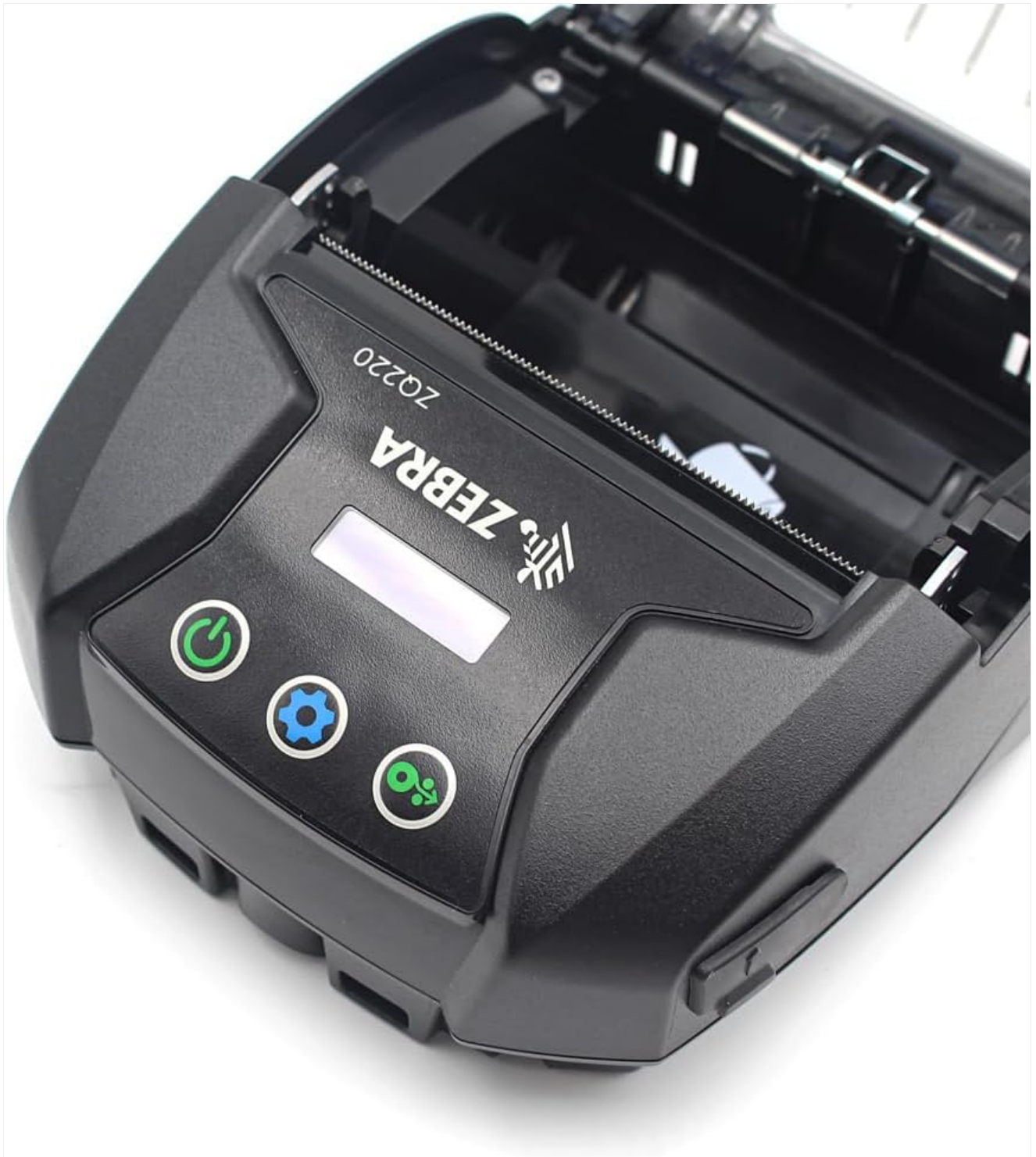
Figure 2: Top view of the ZQ220 printer with the cover open, showing the internal paper compartment.
