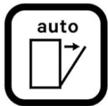
Figure 5.5: The dishwasher door automatically opening slightly at the end of a cycle for enhanced drying.
