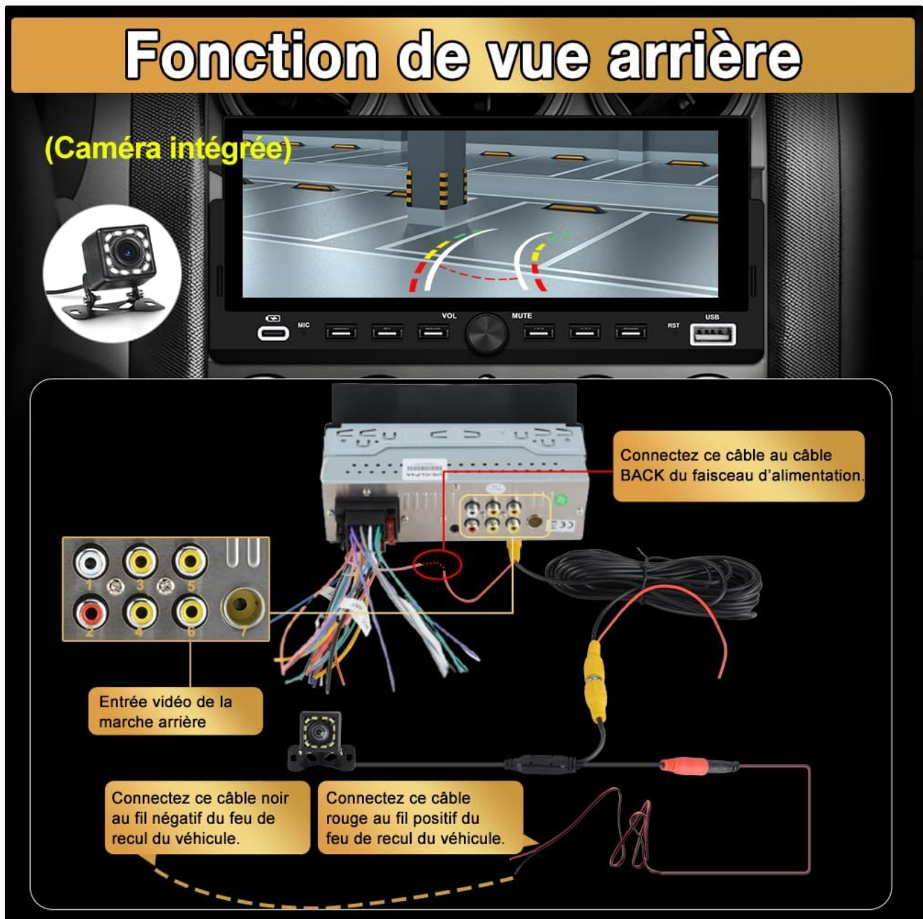
Image: Diagram illustrating the correct wiring for the rearview camera to the car stereo and vehicle's reverse lights.
