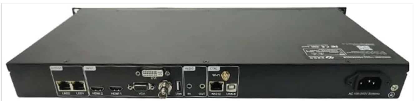
Image 2: Rear view of the EnhanBili HD-VP210H Video Processor. This image shows the back of the unit with various ports. From left to right, there are two LAN ports (LINK1, LINK2), USB, HDMI 1, HDMI 2, DVI, VGA, CVBS, Audio In (3.5mm), Audio Out (3.5mm), Wi-Fi antenna connector, another LAN port (CTRL), and the AC power input (AC 110V~240V).
