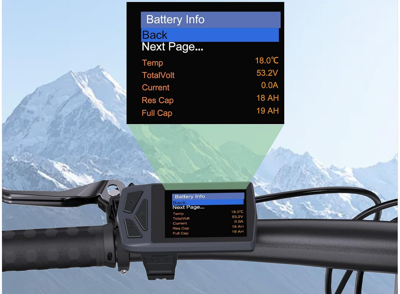
Figure 7: Display screen showing detailed battery information such as temperature, total voltage, current, and capacity.
