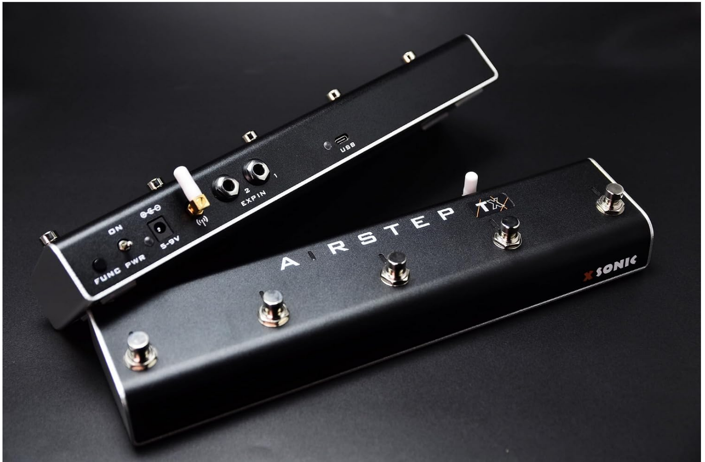
Image: Rear panel of the Airstep TX, highlighting the power input, USB port, and expression pedal inputs for various connections.
