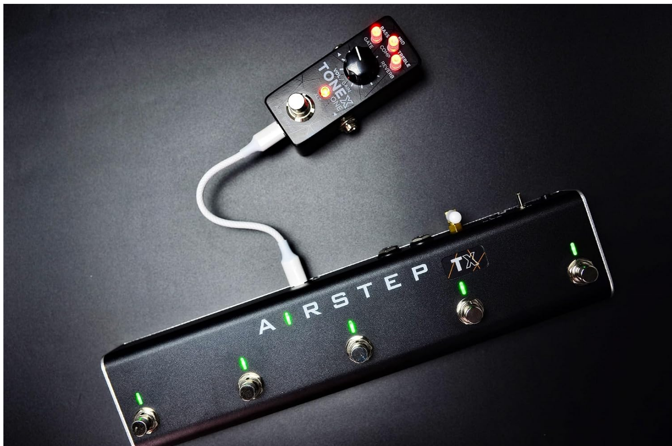
Image: The Airstep TX connected to a TONEX ONE pedal via USB, demonstrating the power and control link.
