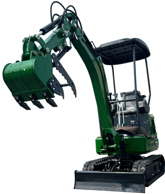
Figure 3.3: Front three-quarter view highlighting the bucket and the non-hydraulic thumb attachment, designed for gripping and moving various materials.
