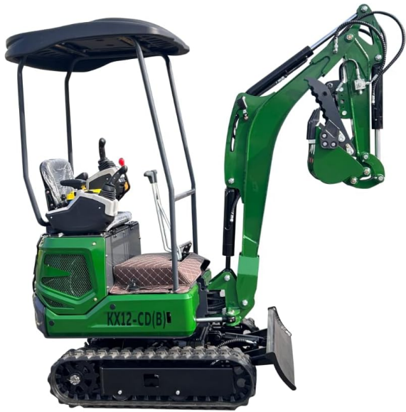
Figure 3.2: Side view of the excavator with the front blade in the lowered position, used for leveling or stabilization. The compact design is evident.
