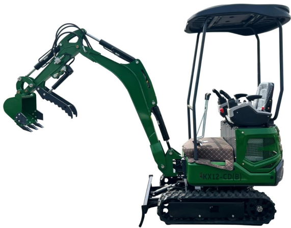
Figure 3.1: Side view of the AGT KX12-CD(B) Mini Excavator, showcasing the main body, tracks, boom, arm, and bucket assembly. The operator's seat and control levers are visible.
