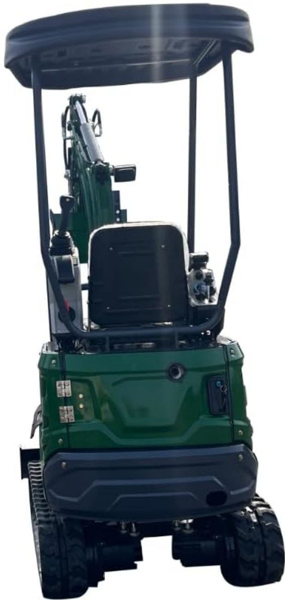
Figure 3.6: Rear view of the mini excavator, showing the counterweight and the overall sturdy construction. The rear lights are also visible.
