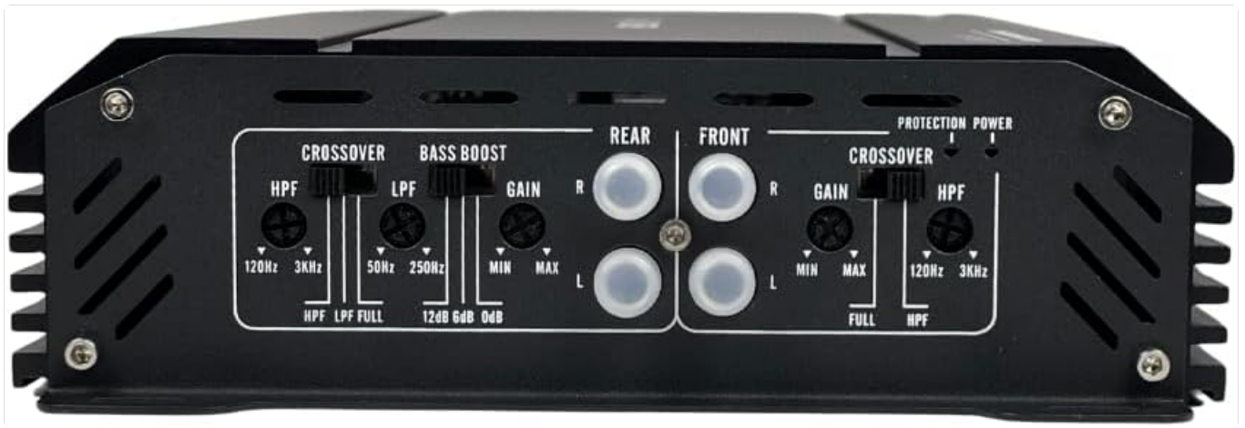
Image: Front panel of the amplifier, showing the control knobs for Crossover (HPF, LPF, FULL), Bass Boost, and Gain for both front and rear channels, along with input RCA jacks.
