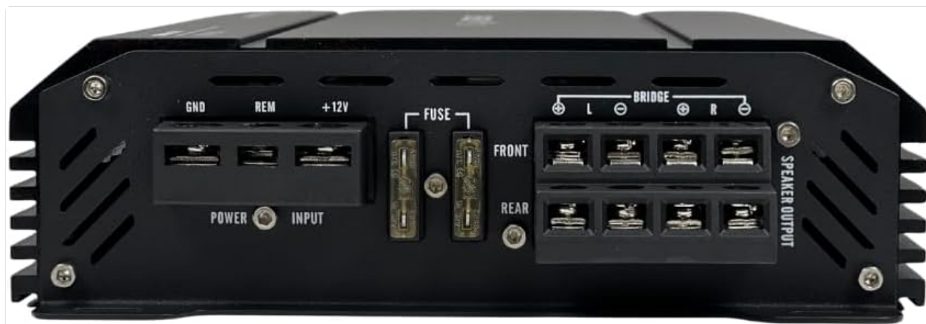
Image: Rear panel of the amplifier, detailing the power input (GND, REM, +12V), fuse slots, and speaker output terminals (L/R for front and rear channels, and bridgeable option).
