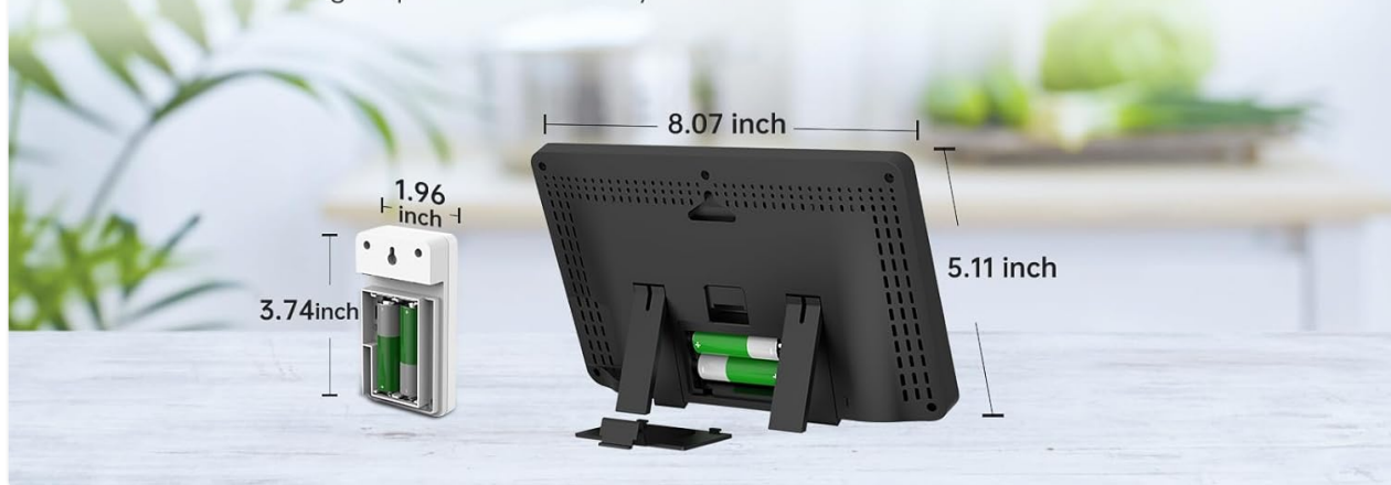
Figure 2.1: Illustration of the two power supply options for the main unit: AC adapter for constant display and batteries for intermittent display.
