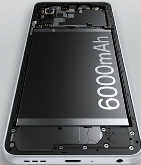
Image: An internal view of the OPPO A5X 5G, highlighting the large 6000mAh battery component.
