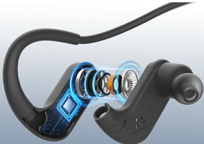
Image: A cutaway view of the in-ear headphones, highlighting the high-quality speaker drivers for rich, full sound.
