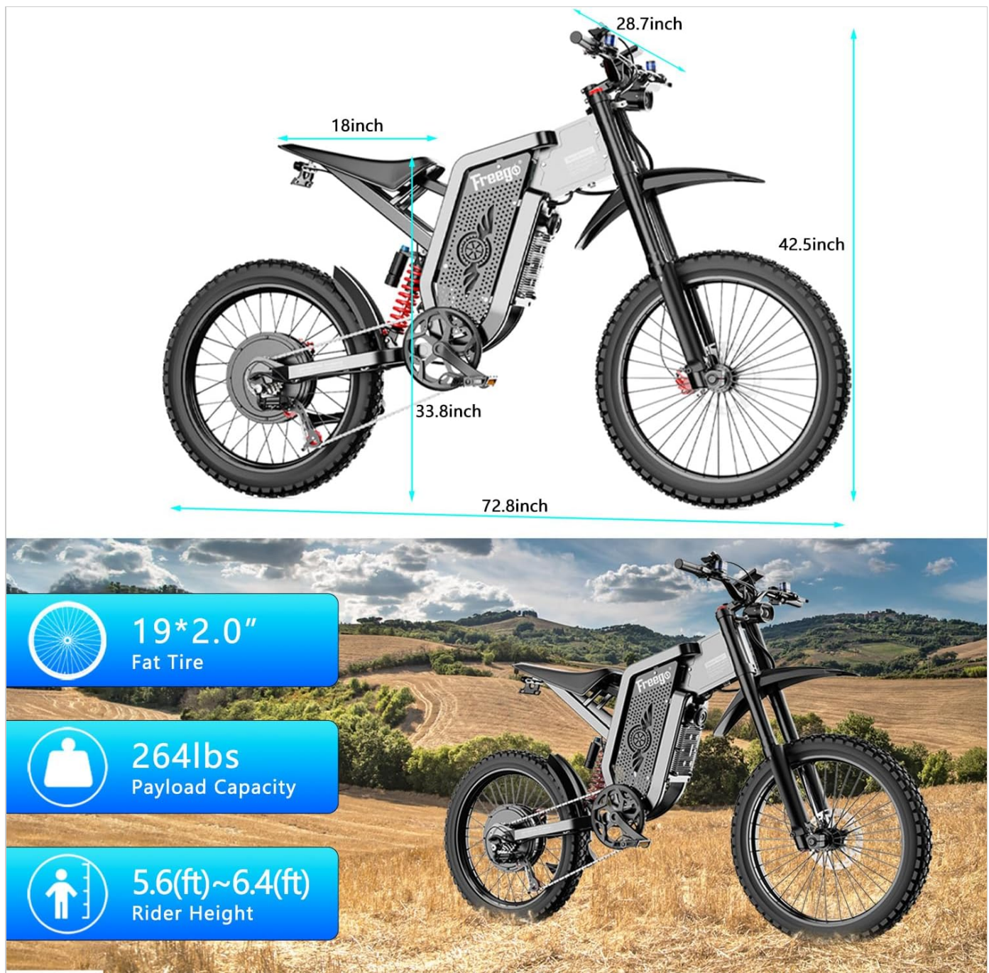
Image 7.1: Visual representation of the Freego X2 dimensions, recommended rider height, ebike weight, and load capacity.
