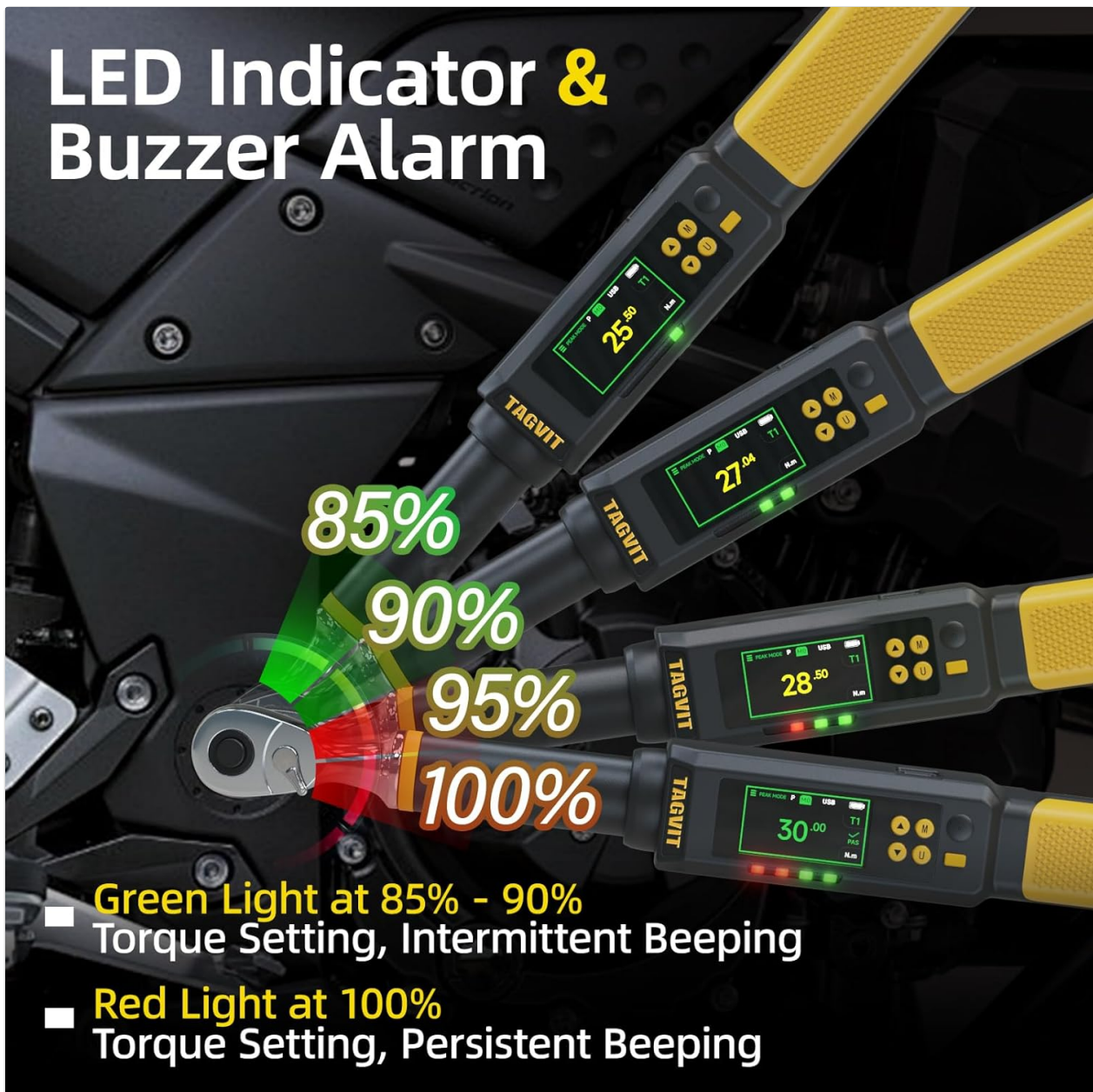
Figure 5.3: Visual representation of the LED indicator and buzzer alarm system, showing green light for approaching torque and red light for target torque reached.
