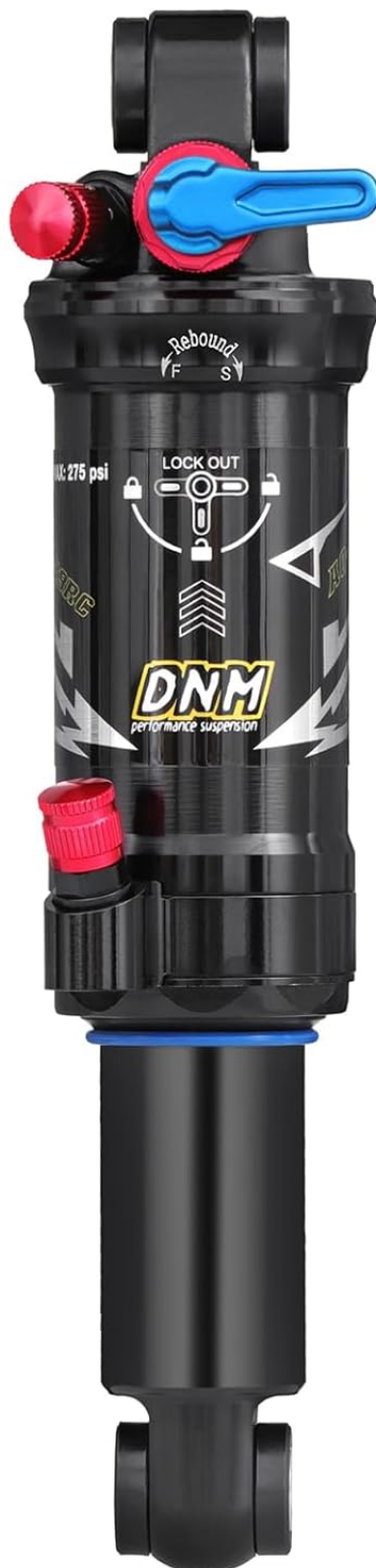
Image 4.2: Visual guide for rebound adjustment. Turning clockwise (S) increases damping for slower rebound, while turning counterclockwise (F) decreases damping for faster rebound.
