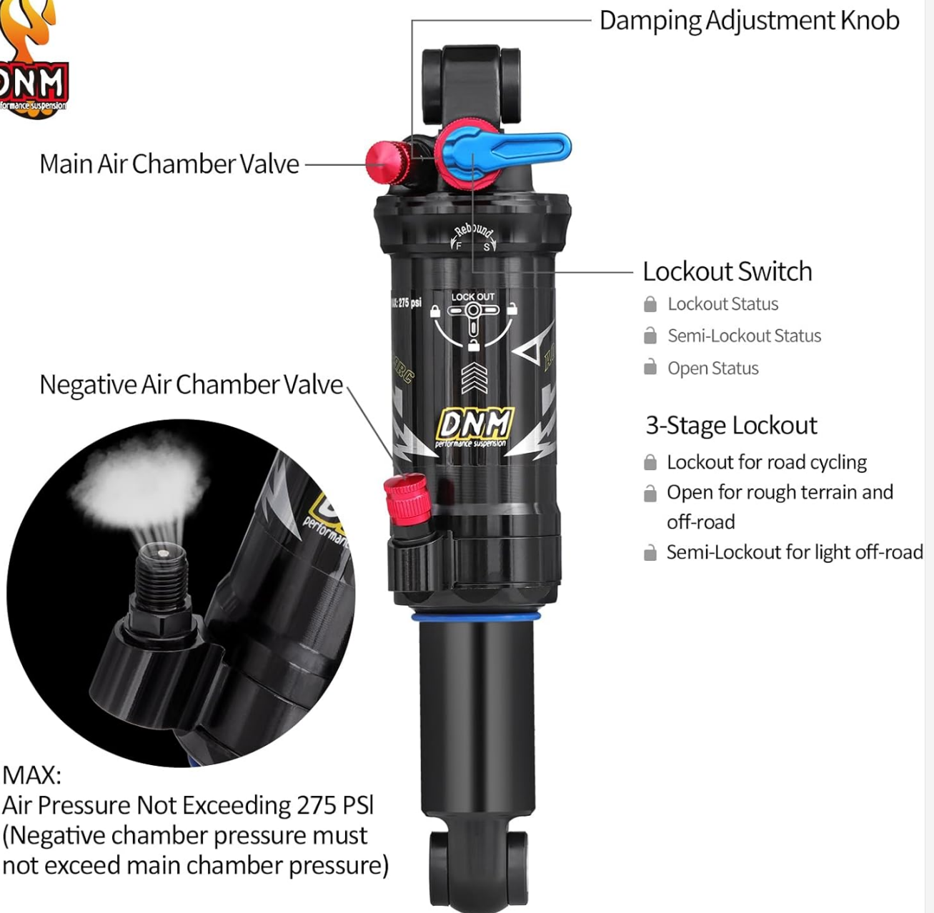
Image 4.1: Labeled diagram of the DNM AO-39RC rear shock, indicating the Damping Adjustment Knob, Main Air Chamber Valve, Negative Air Chamber Valve, and Lockout Switch.
