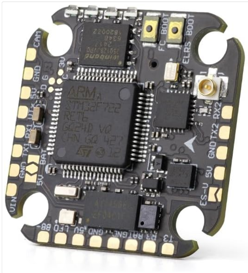
Image: Top view of the HGLRC SPECTER F722 Lite Flight Controller, showing the main MCU, gyroscope, and ELRS module.
