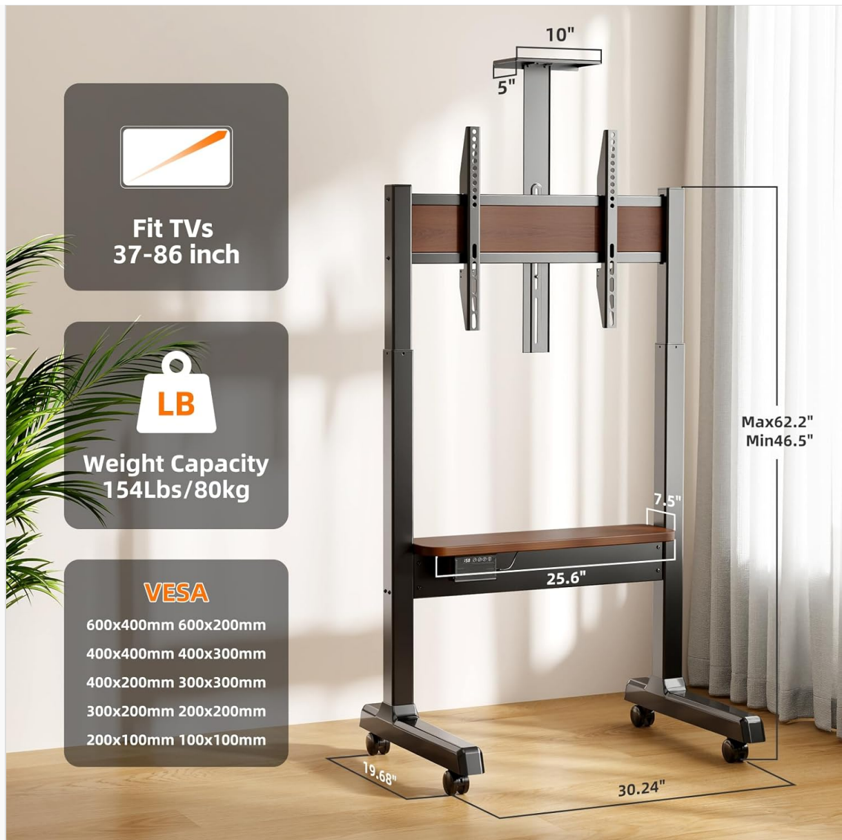
Image: Overview of stand dimensions, VESA compatibility, and weight capacity.
