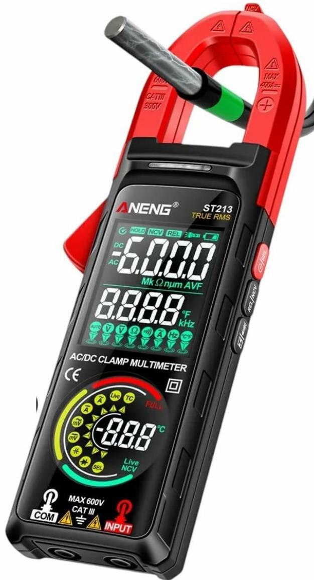
**Figure 2.1:** Front view of the Aneng ST213 Digital Clamp Meter. This image displays the device with its clamp jaw open around a conductor, showing the dual display screen, function dial, and input terminals.
