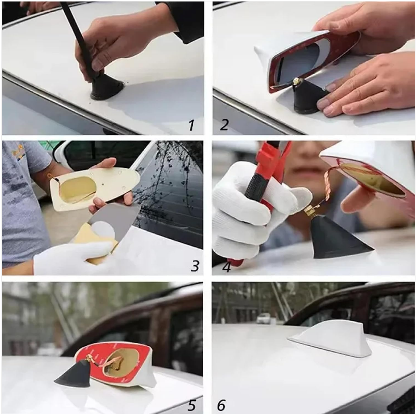
Figure 3.1: Step-by-step visual guide for installing the shark fin antenna. This includes removing the old antenna, connecting the new one, and securing it with adhesive.
