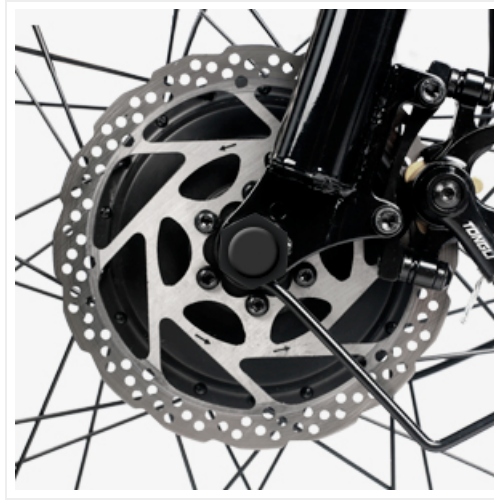
Image: A close-up view of the front disc brake system, illustrating the rotor and caliper for effective stopping power.
