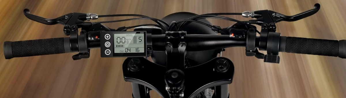
Image: The S866 multi-function LCD display mounted on the handlebars, showing speed, battery level, assist level, and time.
