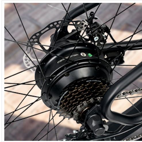
Image: A detailed view of the rear wheel, showing the motor hub and the 21-speed cassette, part of the bike's drivetrain.
