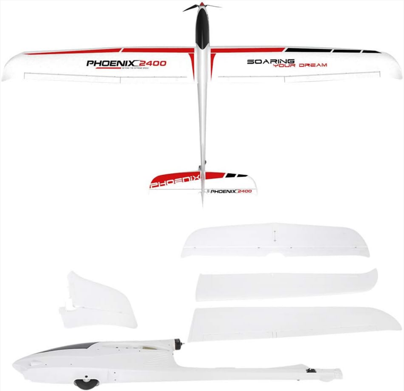
Image 3.1: Overview of the Volantex Phoenix 2400 components, including the fuselage, wing sections, and tail pieces.
