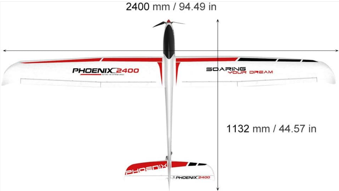
Image 4.1: Dimensional overview of the Phoenix 2400, showing its 2400mm wingspan and 1132mm length.
