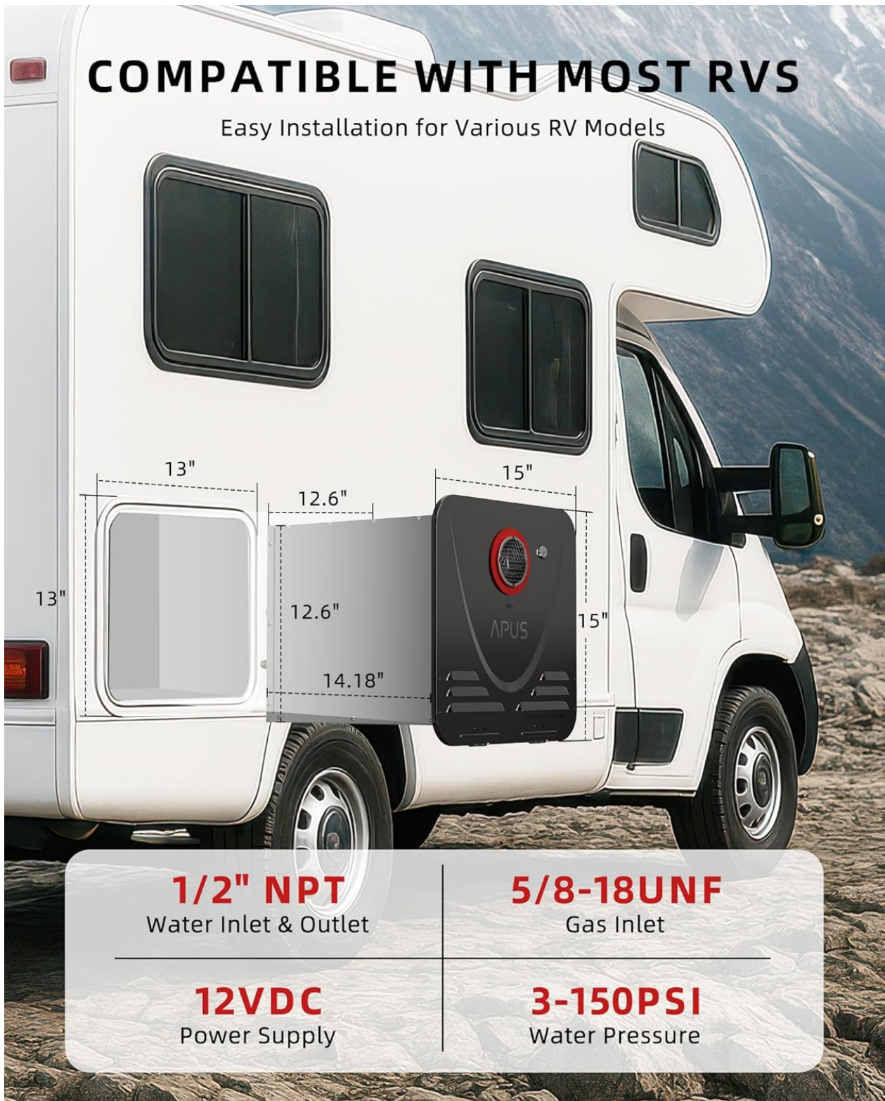
Image 4.1: Dimensions of the APUS RV Tankless Water Heater for installation reference.
