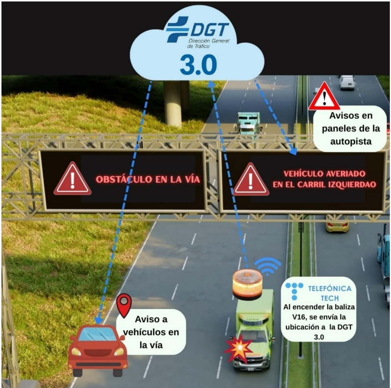
Image: Illustration of the DGT 3.0 system receiving beacon signals and alerting drivers.
