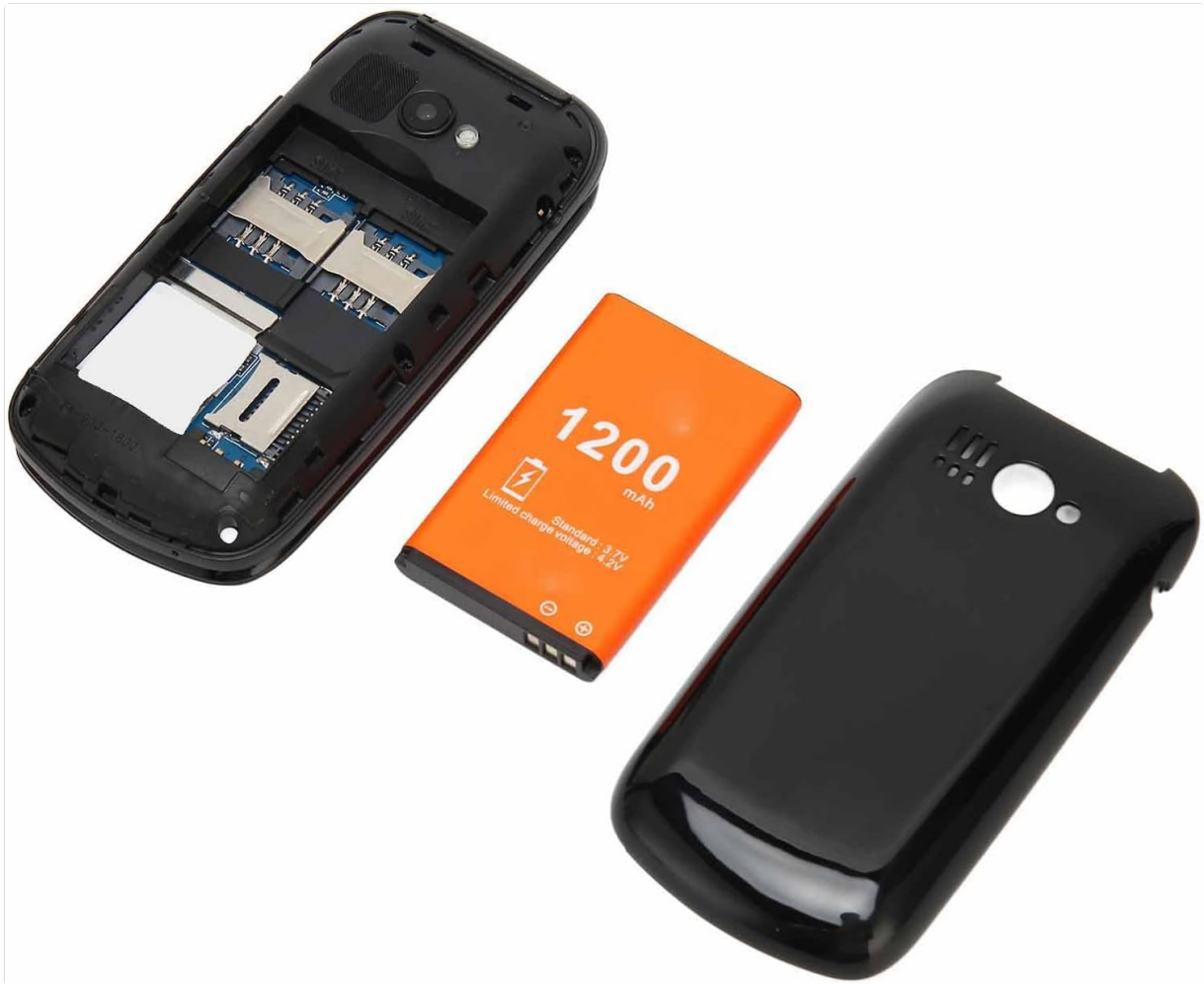
Image: Internal view of the phone showing battery, SIM card, and memory card slots.
