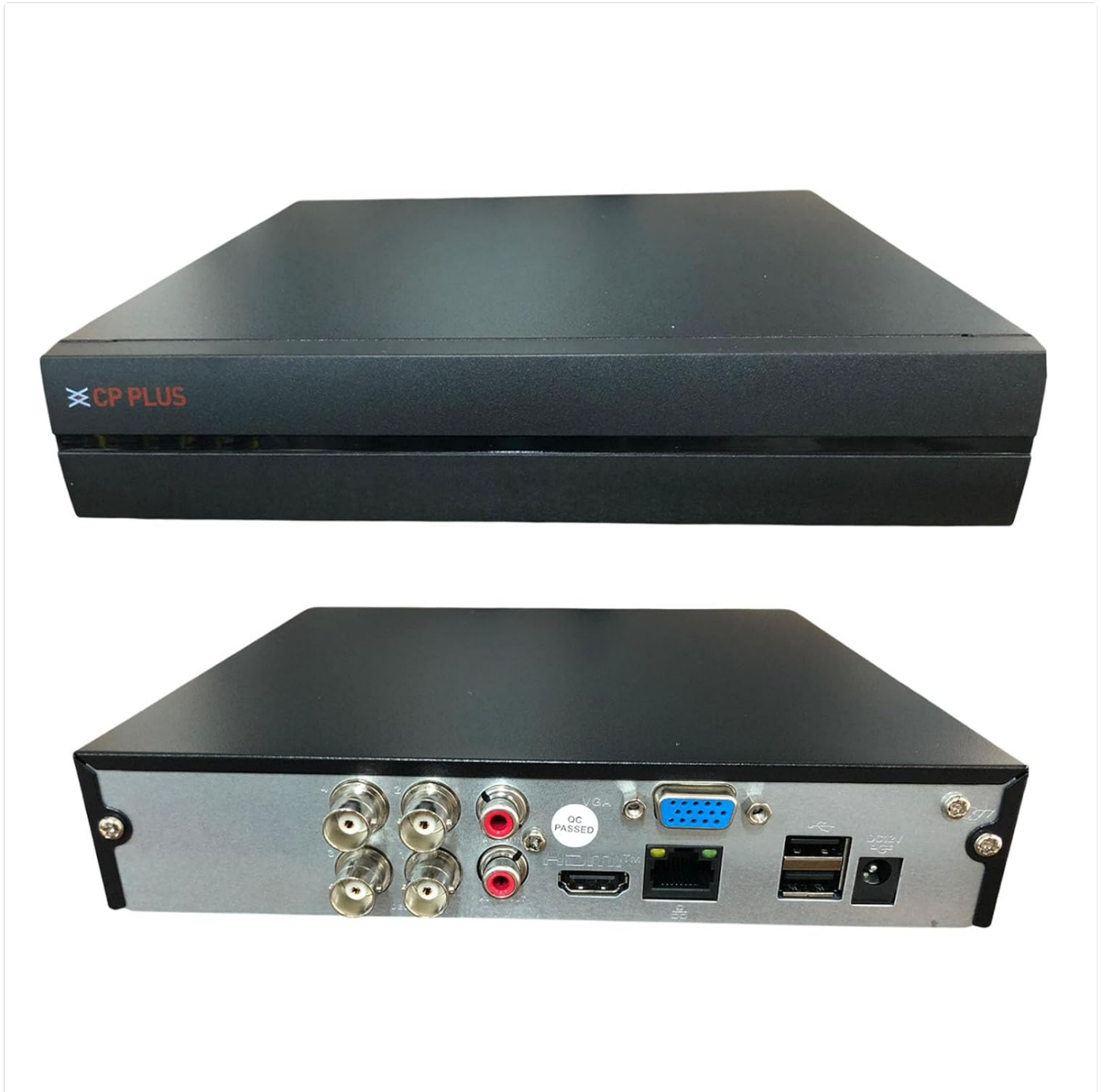
Figure 2: Front and rear panel connections of the DVR, showing BNC inputs, audio ports, HDMI, VGA, Ethernet, USB, and power input.
