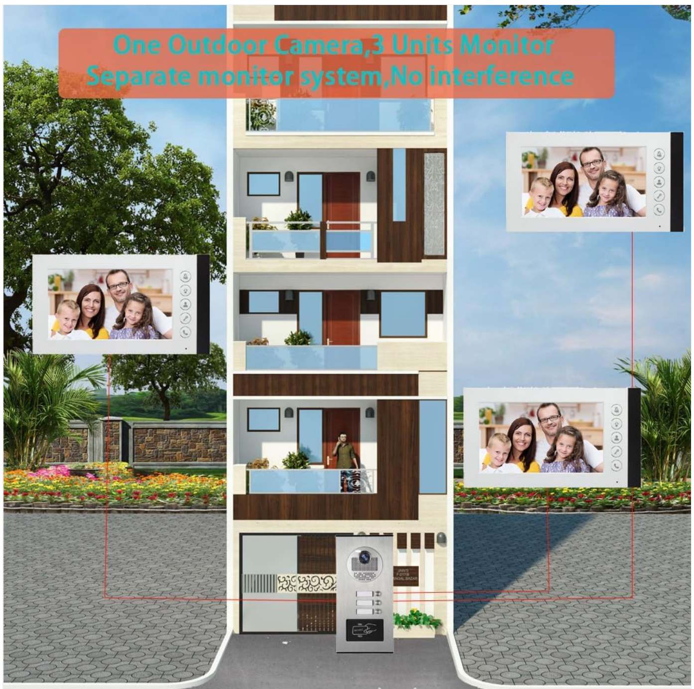
Figure 2.1: Multifamily Intercom System Overview. This image illustrates a typical installation in a multi-story building, showing one outdoor doorbell unit connected to multiple indoor monitors, allowing separate monitoring for each unit without interference.
