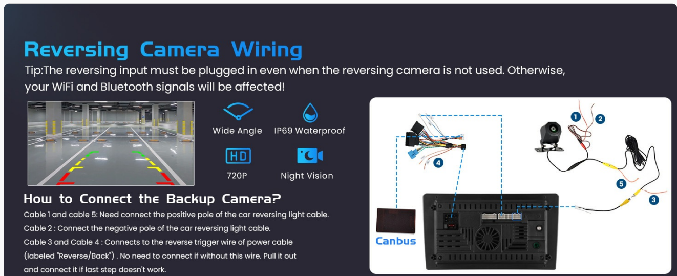
Figure 3: Backup Camera Wiring Diagram.
