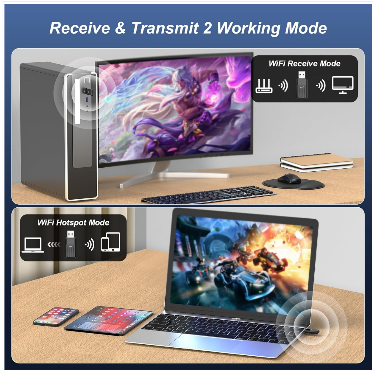
Image 6.1: Diagram illustrating the two working modes: WiFi Receive Mode, where the adapter connects the PC to a router, and WiFi Hotspot Mode, where the PC shares its internet connection with other devices.
