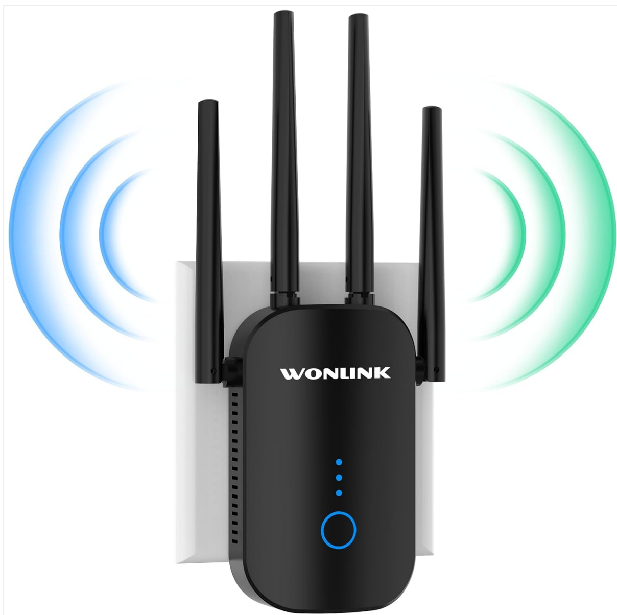
Figure 4.1: Front view of the WONLINK WiFi Extender, showing LED indicators and WPS button.
