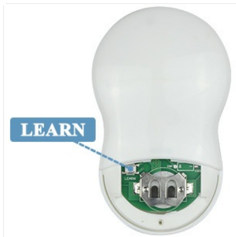
Image: Close-up of the remote control's battery compartment, showing the 'LEARN' button.
