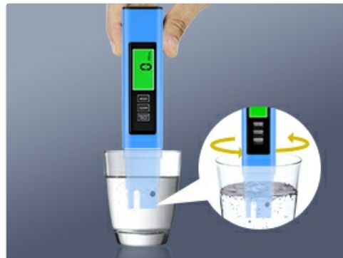
Image 3.2: Gently stirring the meter in the water to ensure accurate and stable readings by removing air bubbles.
