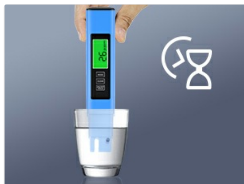
Image 3.3: The TDS meter displaying a stable reading after the probe has been immersed and gently stirred in the water sample.
