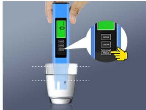
Image 3.1: Proper immersion of the TDS meter probe into a water sample. Ensure the water level does not exceed the indicated immerse line.
