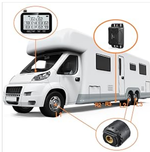
Image 2.3: RV with TPMS Components Diagram. This diagram illustrates the typical placement of the monitor, sensors, and signal booster on an RV.
