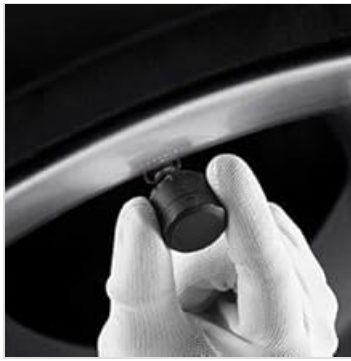
Image 2.2: Sensor Installation. A close-up view of a hand installing a tire pressure sensor onto a valve stem.
