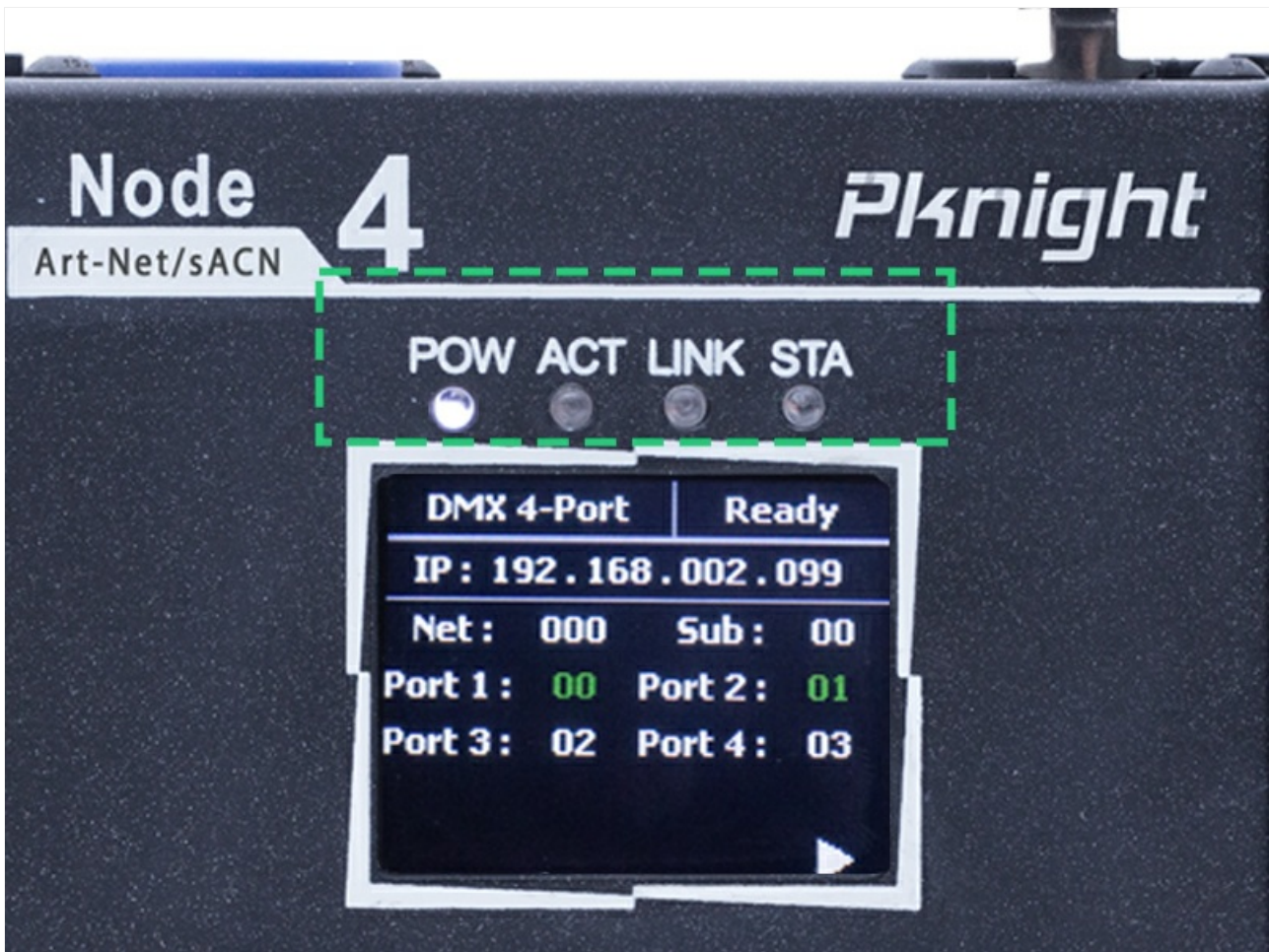
Image: A detailed view of the 1.8-inch color TFT display, which provides real-time information including the device's IP address, Net, Subnet, and the input/output status of each DMX port.
