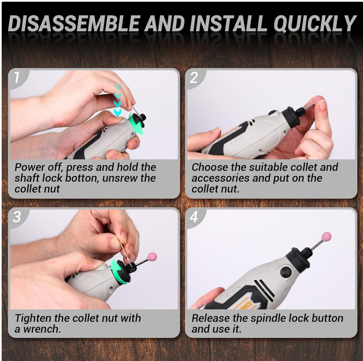
Image 5.1: Step-by-step guide illustrating how to disassemble and install accessories on the rotary tool by using the shaft lock button and collet nut.
