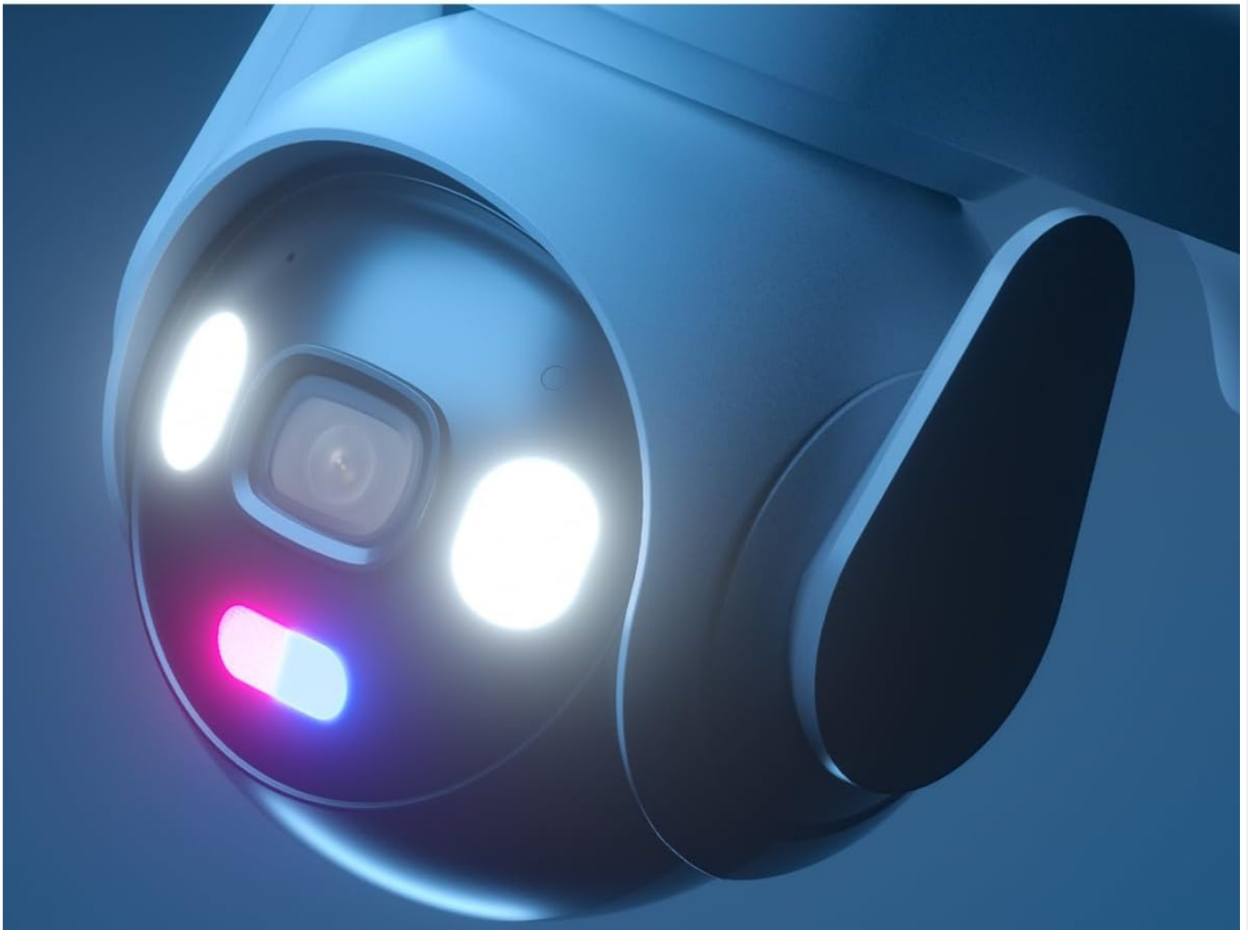
Figure 6: A close-up view of the camera's front, with its red and blue warning lights illuminated. These lights serve as a visual deterrent against unauthorized presence.
